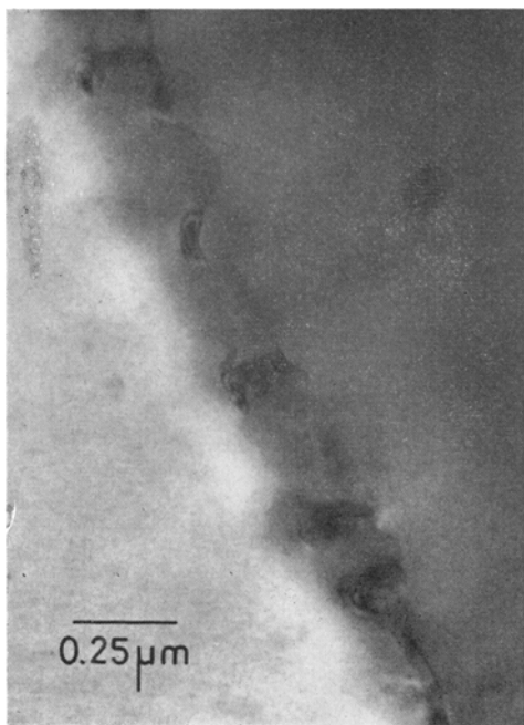
Figure 1 The discontinuous precipitation reaction observed for the solution-treated condition aged for 20 h at 200°C.
