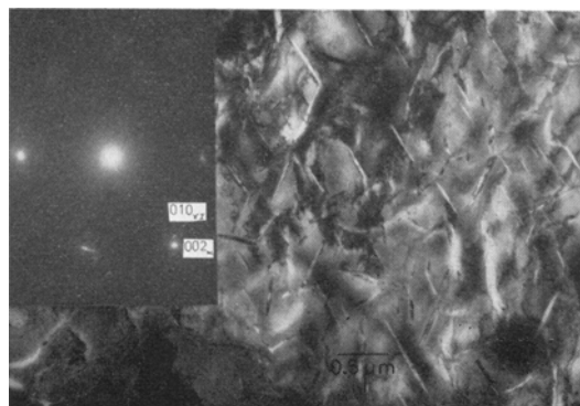
Figure 3 \gamma I precipitates observed for the solution-treated condition aged for 24 h at 425°C. The selected-area diffraction pattern shows \gamma I to have a similar orientation to the continuously precipitated \gamma' .
